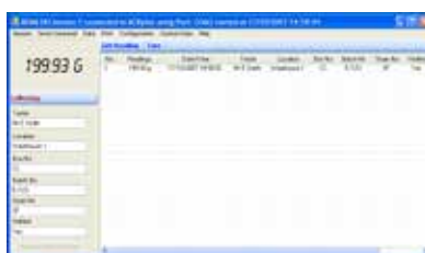
Six user-defined fields are available for custom data entry with each reading. Custom data can be exported with the weighing data.
