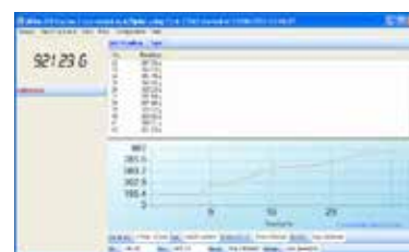
Real time graphing and statistics are easily viewable in the data grid. Balance control buttons let you request data or tare the balance right from the software.
